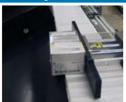
The flexible FAST Sort solution The FAST Sort solution includes all the control hardware and software functionality needed to ensure accurate, consistent and verifiable automated sortation and control. The Windows® based tracking system is efficient and fast, managing hundreds of I/O points while operating at functions on both tilt-tray and conveyor speeds over 600 fpm cross-belt sortation machines. [3 mps].
