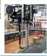
Immediately following label application, a bar code scanner verifies the proper application and label content.
