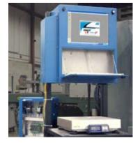
4 Label formatting, printing and application are done on-the-fly by one or more printer-applicators. Item-specific labels are automatically printed and applied to each package.
