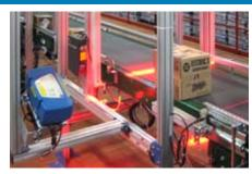
2 FAST Label is configurable to include in-motion weighing; weight is automatically captured and verified against configurable criteria.
